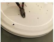
Step 5: Remove the lens and the LED-Board.
