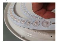
Step 6: An individual light source is removed out of the containing product.
