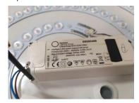
Step 4: Cut off the latch from the lens on the back of the ceiling base.
