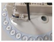
Step 3: Remove the screws from the driver.
