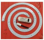
Step 7: Fix a new connection wire to the light source by using electric iron. Take care of the LEDs during this step, do not touch them.
